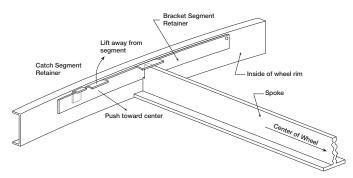
**Important!** Place retainers back in the original position before rotating the energy recovery wheel, otherwise damage to retainer will occur.
